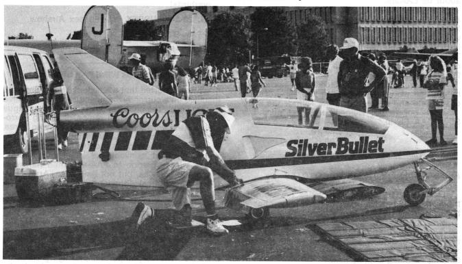
Due to the fact that the Coors Silver Bullet is a jet and consumes copious quantities of fuel, the aircraft is dismantled and placed in a trailer after each show performance for its cross country journey to the next airshow. Photo shows tailfeathers and left wing already removed after completing its routine at the recent Pratt & Whitney Airshow.
