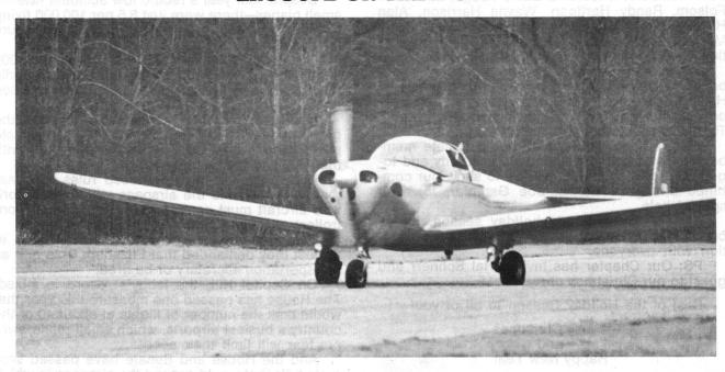
The Seemann-Bullock Ercoupe finally got underway recently. Above photo shows Bob Seemann taxiing the aircraft to the run-up area at Lakeside Airport on November 25, 1987. However, after a short flight an oil leak was discovered in the kidney-shaped oil tank of the Continental 85 resulting in the loss of several quarts of oil. As of this writing it is being repaired so it will be several days before it will be flying again.
