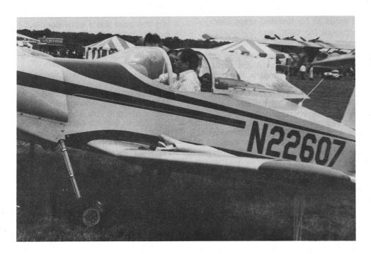
Photo shows Chapter 166 Technical Counselor Joe Gauthier seated in the cockpit of his newly (almost) completed Thorp T-18 at the Pratt & Whitney Aeroservice Airshow in East Hartford this past Fall. As you can see, the landing gear fairings and wheel pants haven't been installed. We understand Joe has flown off his required flight time and is ready for a trip to Sun 'N Fun and of course, Oshkosh.
