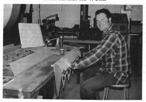
Or should the description read "Craftsman at Hobby"? Photo shows Jim Rowley bending plywood around the leading edge of one of his ailerons for the Acro Sport II he is building. Jim has also done a considerable amount of welding on the various parts for his aircraft, fabricating most of the parts from scratch.—Photo by Jim Rowley
