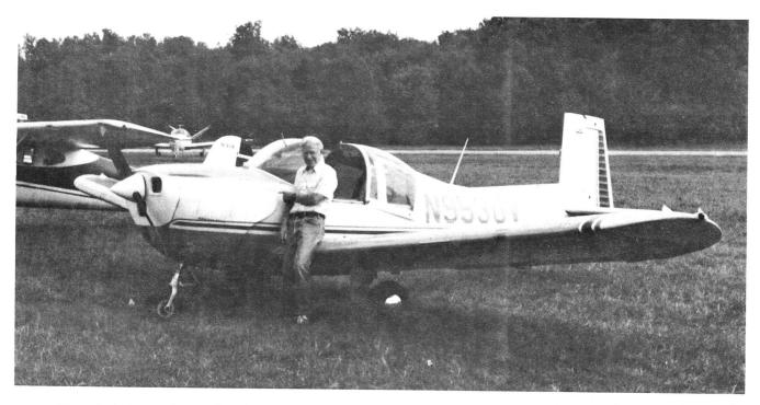
Yours truly is pointing to the builder's name painted on the cowling. Although the name reads "Mooney" the aircraft is an Ercoupe. At one time, Mooney built a number of Ercoupes. (Note the tail assembly).
