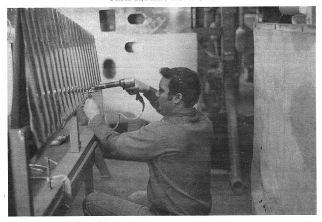
The above scene was taken during a recent trip to Air Service Caravan located on the New Bedford, Mass. Airport to pick up some parts for the Wichawk. The photo shows Joe Bettencourt, of North Dartmouth, Mass., hard at work riveting a Cessna elevator. According to Joe, so much of modern day aircraft work being done by hand necessitates the high cost of any fabricated parts.
