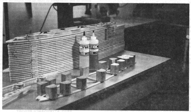
Photo shows stack of wing ribs constructed by Jim Simmons for his new Skybolt project. The 2-part Epoxy glue is shown, together with the lead weights used to clamp the gussets. Ribs are assembled in a jig, glued on one side the first night then removed from the jig and glued on the opposite side the succeeding night. The weights eliminate the need for nails or staples usually used on the gussets.
