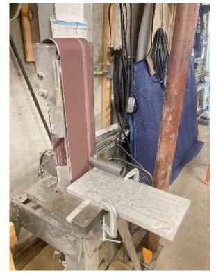
The goal is to rotate the tube around the bolt, slowly feeding the workpiece into the sanding belt.
