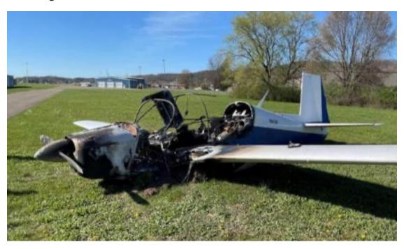
The pilot lifted the airplane cover and saw that a fire had started. The pilot exited the airplane and unsuccessfully attempted to remove the airplane cover, which was on fire. The fire eventually consumed most of the cockpit area (including the battery pack itself) and substantially damaged both wings. (Mark)
