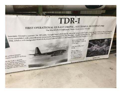
field given the long runways. He said no but it was the site of a top secret project during the war - a drone aircraft that carried a 2000 pound bomb. An operator in another aircraft flew the drone using radio control and a television camera mounted in the drone. It was made of wood and tubing from the Schwinn bicycle company, locat-
