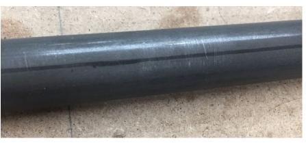
I just slip the rolled template over the tube and trace the cope outline. Just a little work with a cutoff wheel in a die grinder to remove the unwanted material and you're just about there.
