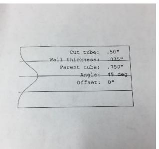
My next step is to take a Sharpie marker and while laying the tube and marker on the table, drag the marker down the tube on both ends giving you a common centerline. This line will be used to "clock" the template. The centerline will also make a common reference for the other side assuming that the other end of the tubing will need some sort of cope as well.
